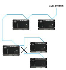
(2) Communication connection between Modbus Gateway(Pro) and air
