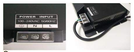
**U**Notice! Power cord should be secured with the equipped wire clip, as shown in the figure.
