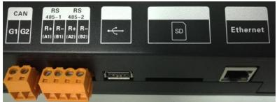
CAN communication interface: It is connected to air conditioner through
